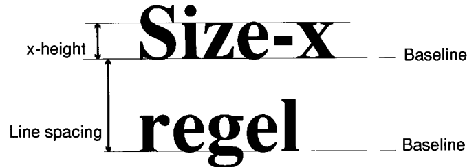
Figure 3. x-height and line spacing can be used to measure typographic dimensions in printed documents.
